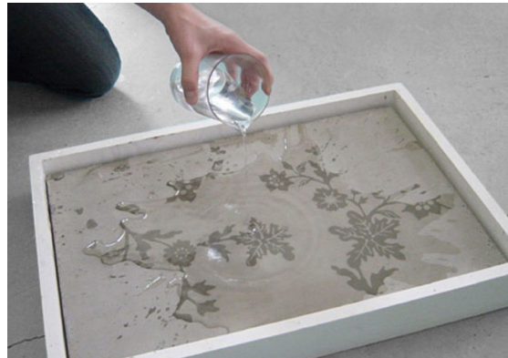
Bio-based self-healing concrete reacts to water
