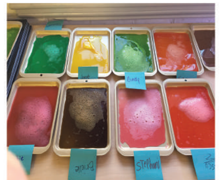
Image: Students' bioplastic (which they dyed using a drop or two of food coloring) cools in trays by the window.
