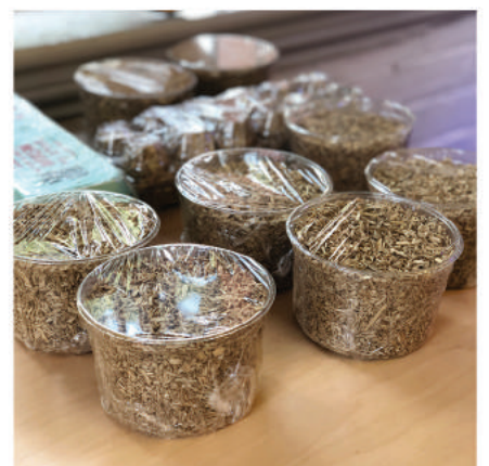
Image: Packed mycelium molds, inoculated and ready to grow over the following two weeks.
